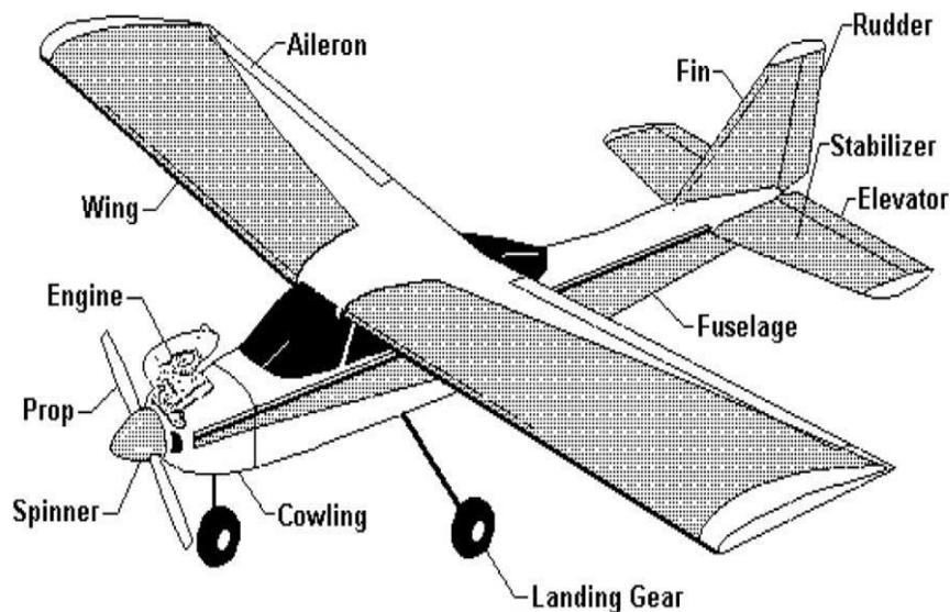
**Aileron:** The moveable portion of the wing which causes a change about the roll axis.
