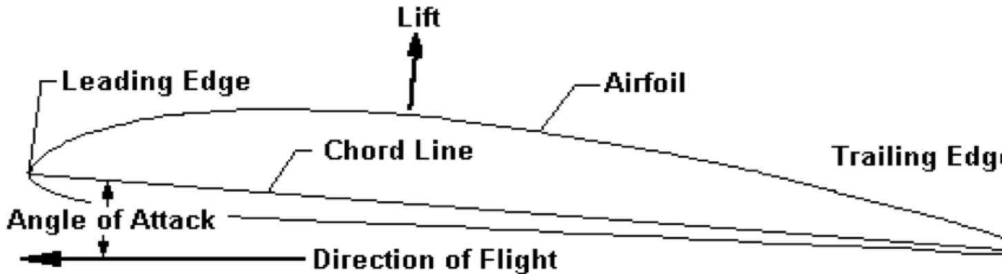
Lift increases as the velocity of the air passing over the wing increases, or as the angle of attack increases, as long as the flow of air over the wing remains smooth. Actual flight is attained when the force of the lift equals weight.
