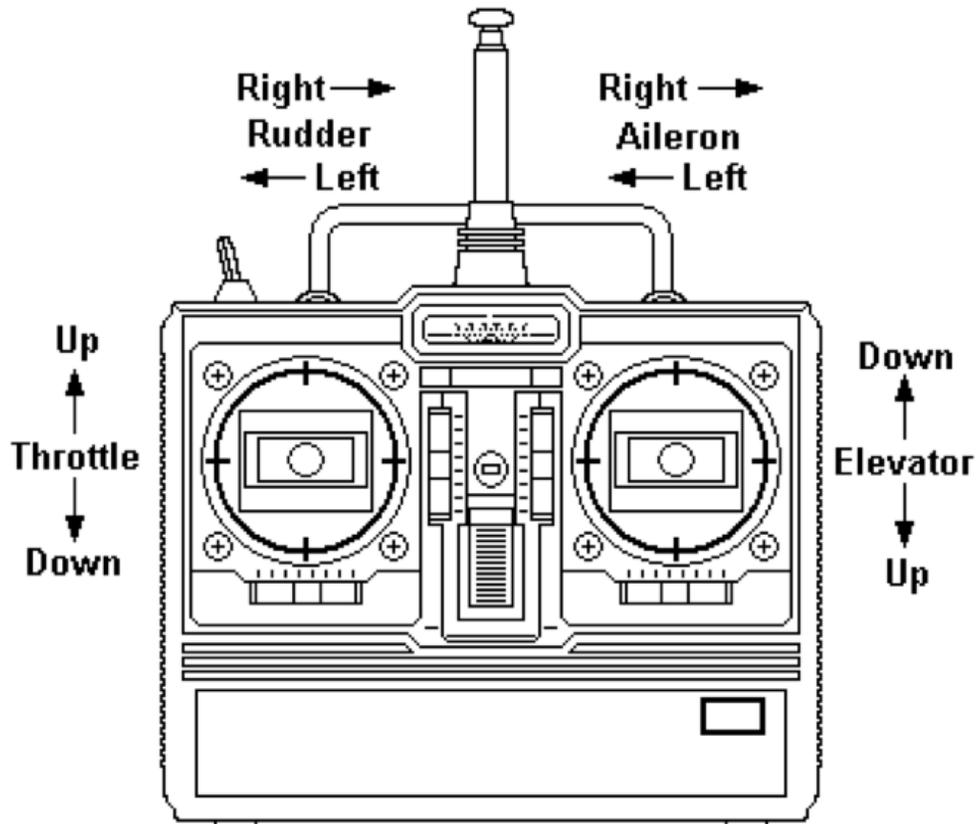
This is a typical layout of the transmitter and its functions. Newer radios have an infinite number of changes and settings that can be made
